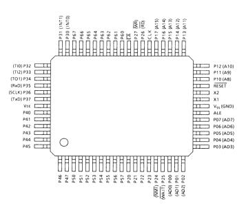
Figure 2.1 (2). Pin Assignment (Flat Package)
