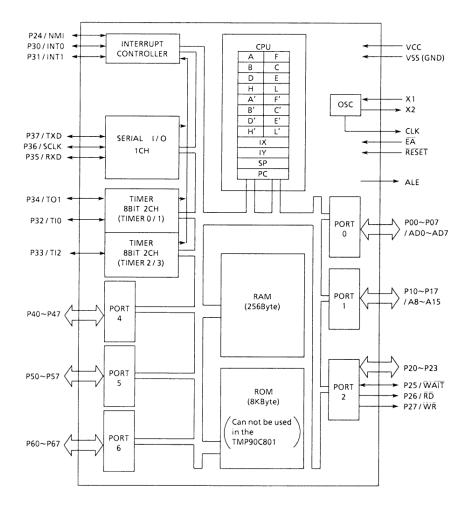
Figure 1. TMP90C800 Block Diagram
